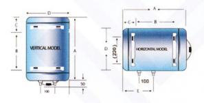
Max. Working Pressure: 0.8 MPa Safety valve Setting: 8 Bar + / - 0.5 Bar
